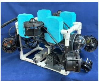
The claw is 3D-printed out of PLA plastic not including the motor and gears.
