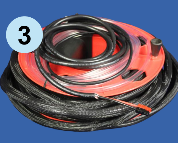
Above: The ROV's four component tether, held in an expandable braided sleeve.
